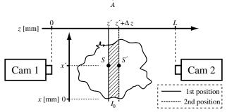
Fig. 1. Schematic of the detection arrangement for dual SLIPI. Two cameras, positioned at  $\pm 90^{\circ}$ , are used for the two SLIPI measurements. The dashed region between the two laser sheets indicate the probed volume over which the average extinction coefficient is calculated. The laser sheets propagate along the *x* direction.
