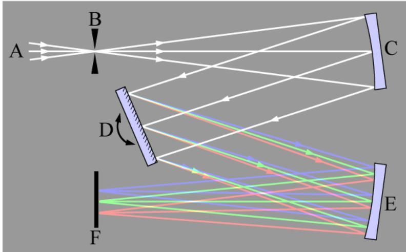
Figure 1: *The basic layout of a Czerny-Turner spectrometer. In the figure, A marks the incoming light. B is the entrance slit. C is the first collimating mirror. D is the reflection grating. E is the second collimating mirror. F is the location of the CCD-chip detector. Source: [4] (Modified)*
