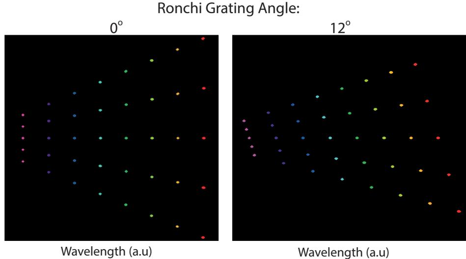
Figure 11: *FRED* simulation results of a spectrum from a light source with eight evenly spaced spectral components in a system where  $x$  is the horizontal axis in the plane of the grating,  $y$  is the vertical axis in the plane of the grating and  $z$  is the axis through the grating: (a) - The grating oriented perpendicular to a collimated beam line, (b) - The grating rotated  $12^\circ$  around the  $z$ -axis.
