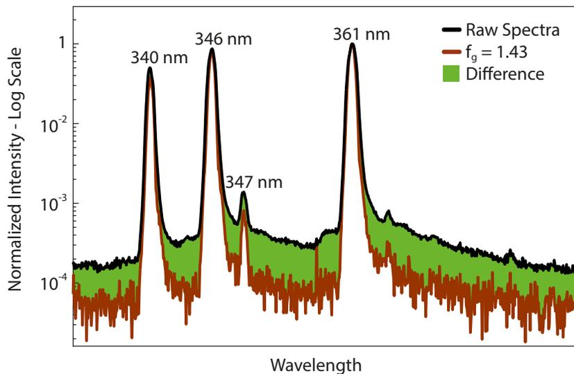
Figure 6: *The difference (green) between a raw emission spectrum (black) and the PS spectrum with the highest Ronchi grating frequency tested (brown) displayed in a lin-log plot.*
