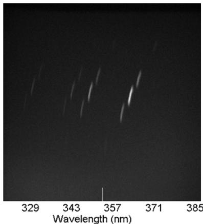
Figure 10: *The detector screen on the spectrometer when a Ronchi grating is introduced into the collimated beam inside the spectrometer. The image displays the hardware Fourier transform of the Cd atomic spectrum with an intense middle stray light peak and one signal peak on each side.*
