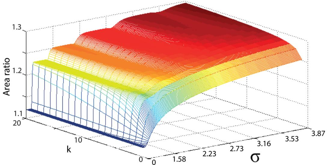
Figure 7: *The area ratio between raw spectrum and PS spectrum of one spectral peak as a function of the filter function width  $\sigma$  and exponent  $k$ . Plateaus of stability are observed around specific  $\sigma$  as long as  $k$  is sufficiently large. Generally, the results show that decreasing  $\sigma$  improves stray light suppression.*
