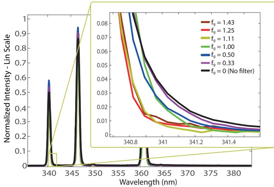
Figure 5: *Seven Cd spectra on a lin-lin scale; one raw spectrum and six PS-spectra. All PS-spectra, each with its own Ronchi grating frequency, (specified in the top right of the plot) have lower levels of stray light compared to the raw spectrum. The results further show that a higher Ronchi grating frequency leads to improved stray light suppression.*
