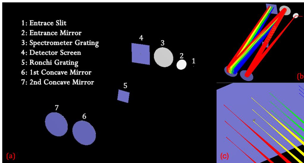
Figure 4: (a) *The replica of a spectrometer created in FRED, with optical components labeled.* (b) *The system after ray-tracing has been done, with rays displayed.* (c) *A close-up image of the detector screen. Four different wavelengths can be seen (Blue, Green, Yellow and Red) as well as the diffraction pattern created by the Ronchi grating in each wavelength.*
