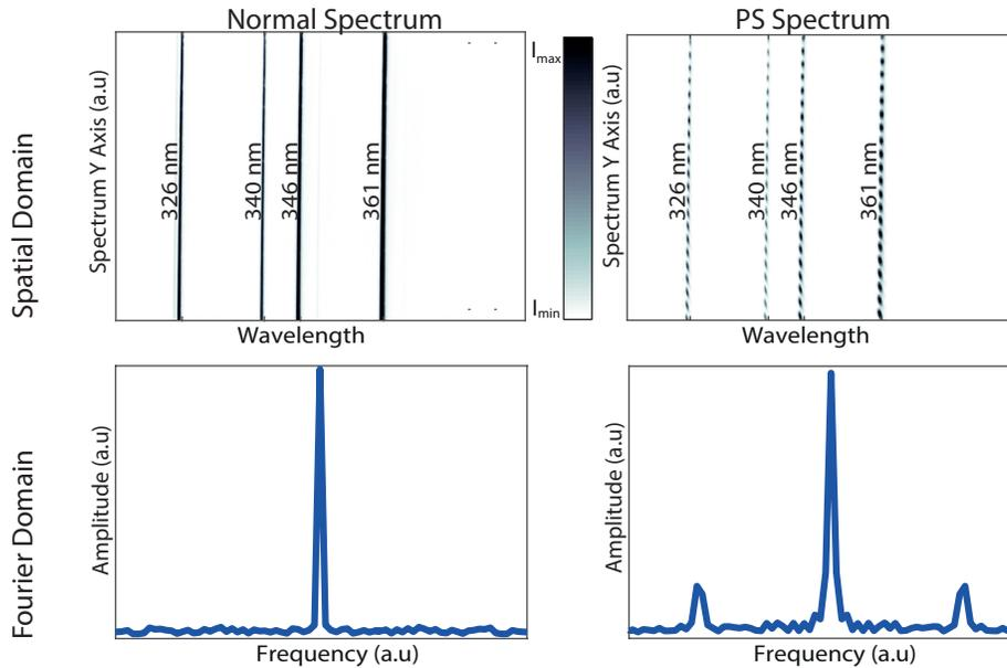
Figure 2: *Cadmium emission spectra, 314.58 nm – 385.49 nm. A regular spectrum (left) and a spectrum affected by a Ronchi grating (right) with their corresponding 1D Fourier spectra. On the right the mirroring Fourier peaks resulting from the introduction of a Ronchi grating are easily distinguishable.*
